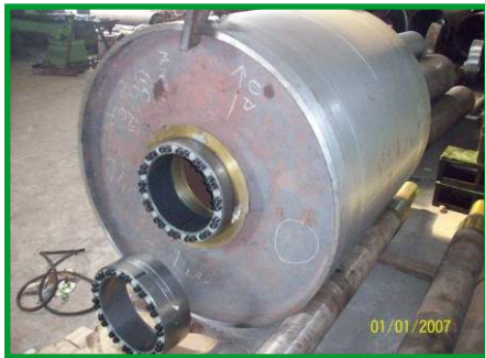
CONVEYOR PULLEY WITH RING FEEDER
